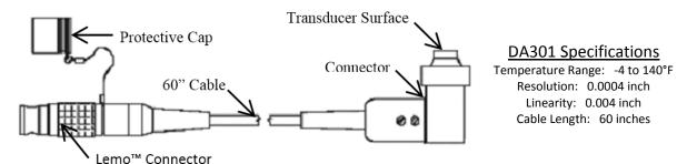
The EESiFlo DA301 Wall Thickness Transducer is specifically designed to provide accurate pipe wall thickness measurements for the EESiFlo 6000 Series Dual Mode, Dual Channel Portable Ultrasonic Flow Meter. Following are simplified instructions for its installation and use:
